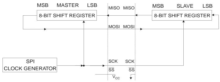
Figure 8. SPI transfer Format with CPHA = 0
