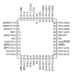
Port 0 also receives the code bytes during Flash programming and outputs the code bytes during program verification. External pullups are required during program verification.
